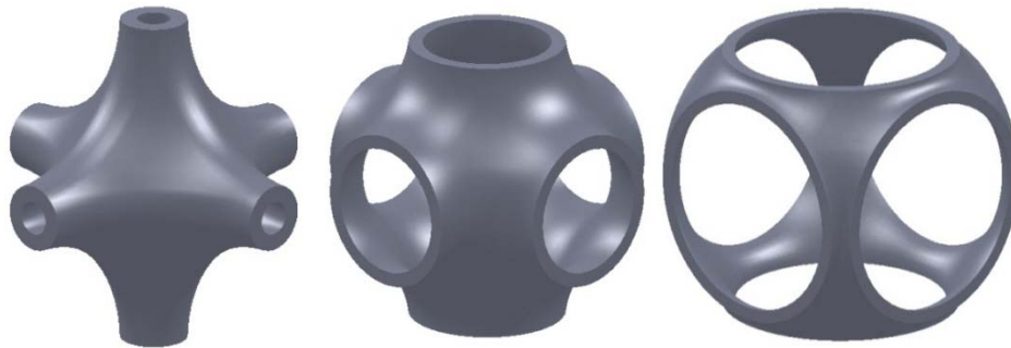
Figure 3.15 – P-minimal surfaces obtained through radius variation with constant surface thickness.
