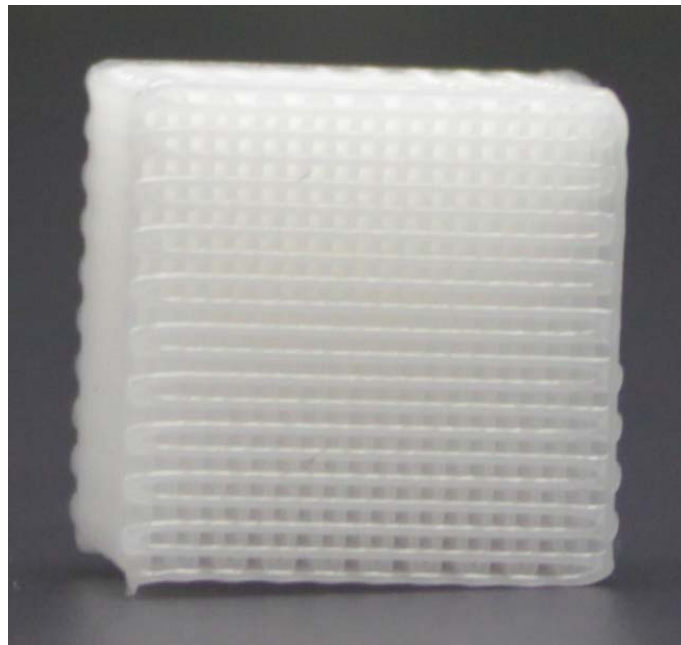
Figure 3.8 – Poly( \epsilon -caprolactone) scaffold with a 0/90 ^{\circ} lay-down pattern.
