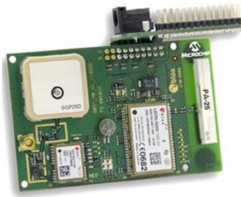
Figura 5.2 - *Machine-To-Machine (M2M) PICTail Daughter Board*.
