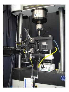
Figure 8.10 - Universal tensile machine adapted to shear tests from the LIMATB, University of South Brittany.
