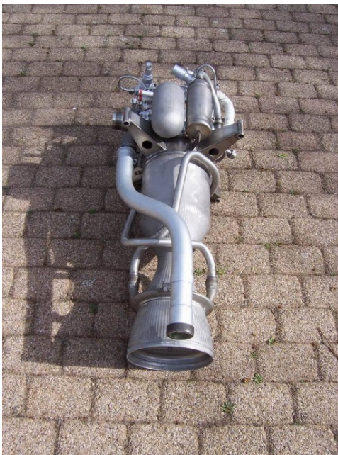
Figure 6.5: Liquid sustainer motor (left) of the russian S-75 missile (right).
