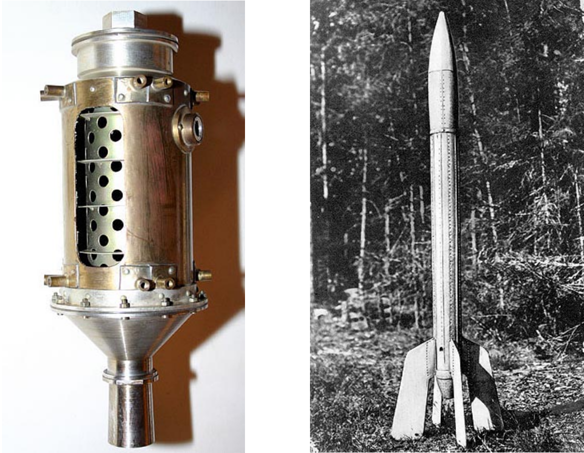
Figure 6: GIRD 09 combustion chamber (left) and complete rocket (right).
