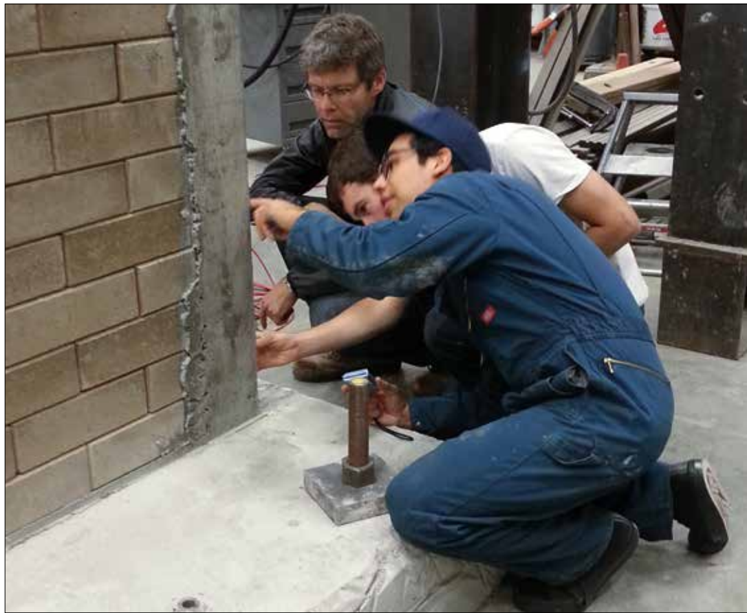
ARCE faculty member Peter Laursen assists civil engineering student Nick Kennedy (center) and graduate student Ivan Castro with the testing of their compressed earth block wall.
