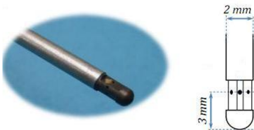
Figure 1. View of the directional probe
