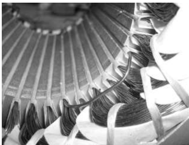
Fig. 10 Stator of rewound PMSM with additional turns (only one can be seen in the figure)
