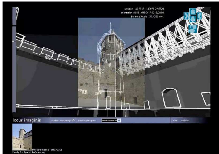
Fig. 5. Manual spatial referencing of images. By means of the keyboard and the buttons of the interface, the user can displace and rotate the navigation camera on which is projected the 2D plane of the image to be positioned in space.
