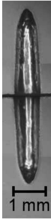
FIG. 8. Optical image of two complementary half-holes revealed by DODO technique.
