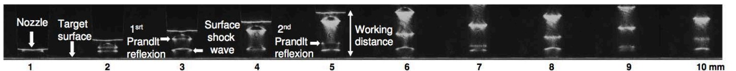
FIG. 5. Strioscopic images of the target surface for several working distances (WD) in millimeters with a 2 bars nozzle pressure.
