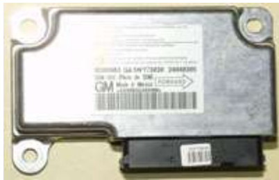
Figure 1 Sensing Diagnostic Module Housing an Event Data Recorder [2]
