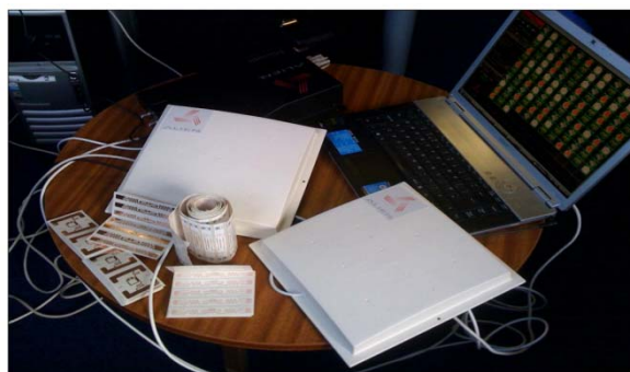
Figure 5 - Passive RFID equipment with corresponding antennas
