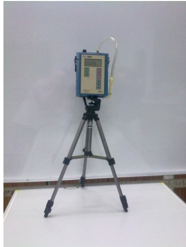
Figure 4. A direct reading instrument using 90 degree light scattering for measuring dust/particulate matters (range from 0.1 to 10 microns particle sizes) in area sampling
