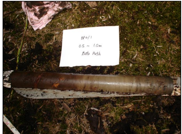
Fig. 3 Peat auger with sampled organic soil
