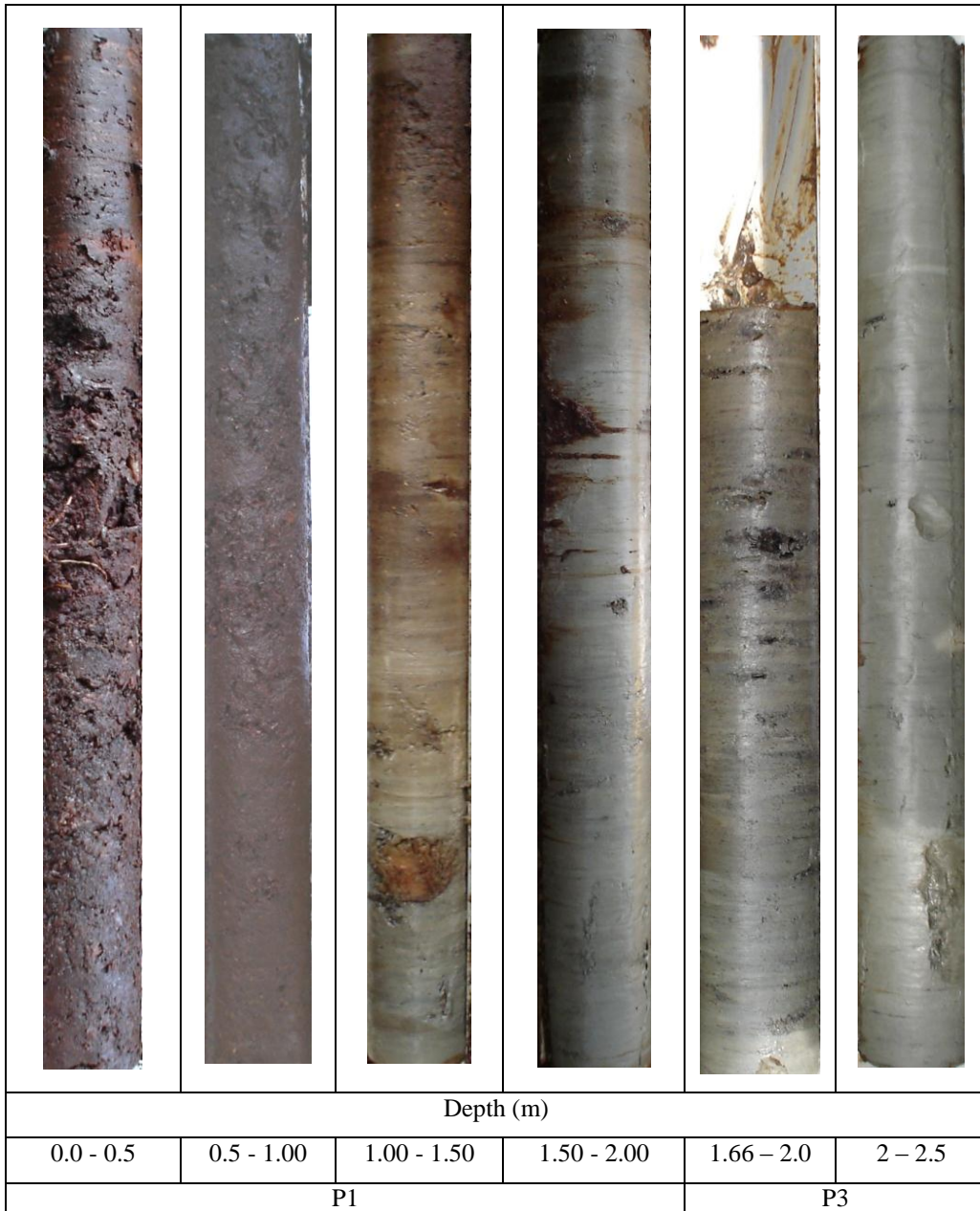
Fig. 5 Photographic record of subsurface layer at Parit Nipah, Batu Pahat
