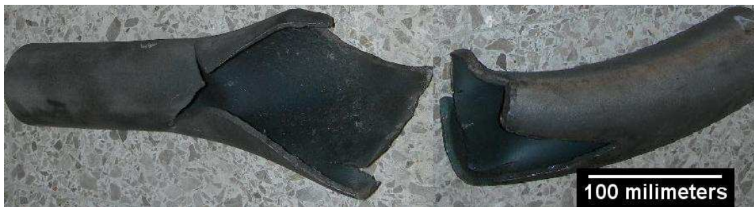
Fig 2 : Digital camera image of fishmouth appearance that catastrophically fractured apart due to high pressure.
