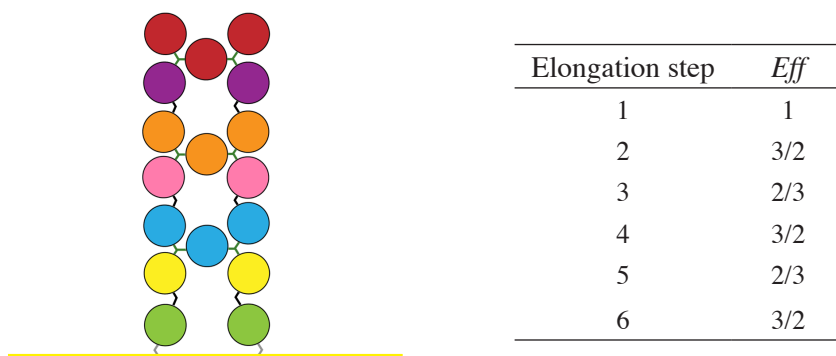
Figure 18 Schematic representation of a growth scenario for the SbS assembly of SAv with alternating ligand construct. SAv was represented as spheres for convenience purposes. Each elongation step of SAv was colored differently and the Eff values expected for each step appear in the above table.
