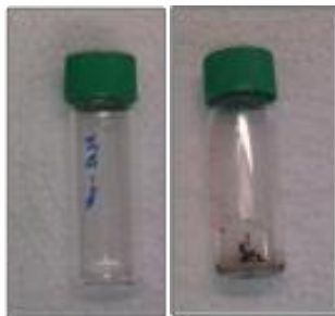
Figure 46. Pictures of aldehyde terminated (right side) and hydroxyl terminated (left side) polymer after the Tollen's test
