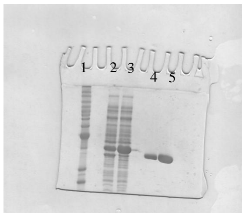
Figure.44. Purity analysis of OmpF by 12% SDS-PAGE. Ladder (1); pre-extracted OmpF (2, 3); diluted OmpF (0.5 mg/ml) (4); concentrated OmpF (1.7 mg/ml) (5).
