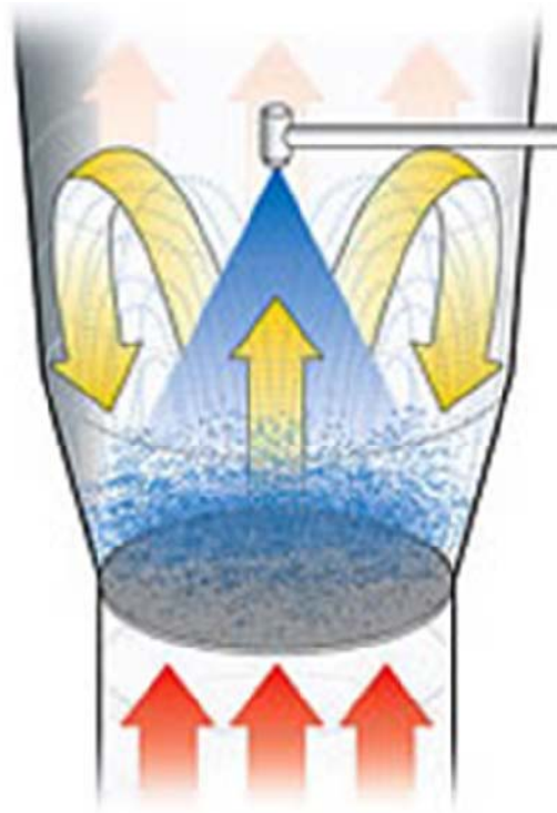
Figure 2: Top spray granulation in fluid bed
