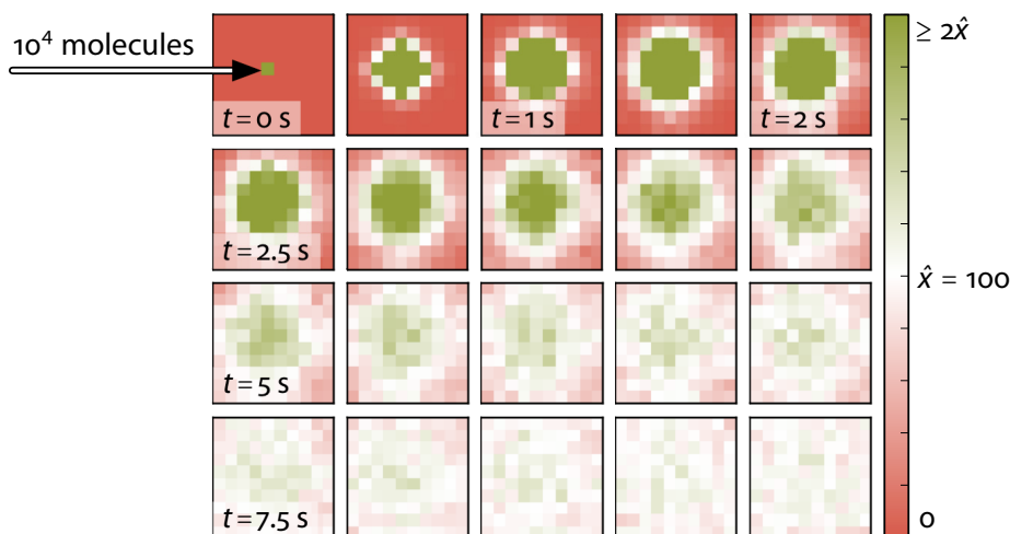
Figure 5.9 OMNeT++ simulation of Disperser : Series of snapshots showing the deviation from the average in a toroidal topology of 100 nodes.
