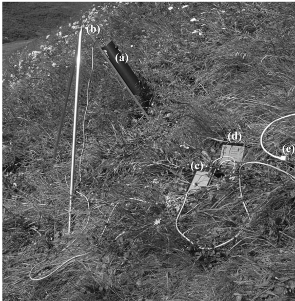
Figure 5.2: NaI detector system with its components: (a) detector, (b) pole, (c) control unit, (d) battery and (e) interface to pocket PC.
