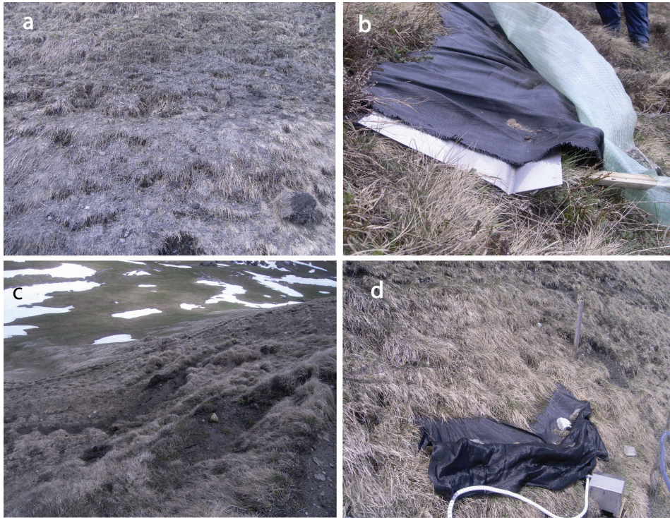
Figure 2.8: Detached soil on the ground after Winter 2007/2008 (upper figure, left side) and sediment trap on plot pawo3 without eroded material (lower figure and figure on right side), some meters away from detached material.
