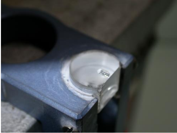
Fig. 4.26. Installation of the specimen on the glass mount of the tripod for the second stage of polishing
