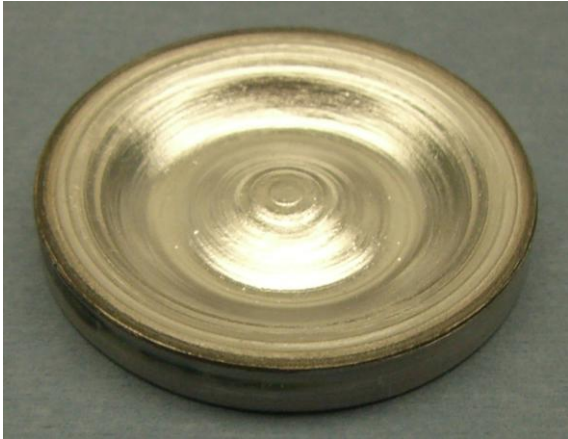
Fig. 3.12. "Racetrack" on a used magnetron-sputtering aluminum target
