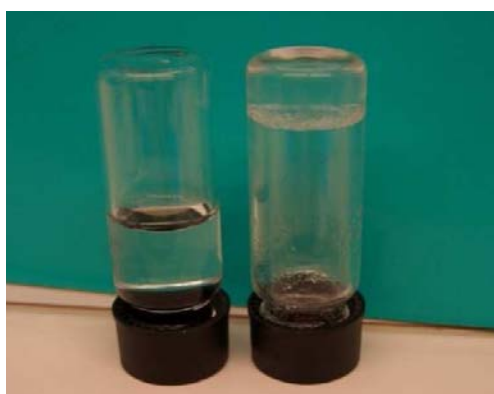
Figure 7: Example of an organogel. Left vial: n-butanol without gelator; Right vial: n-butanol gel with ZVVVOMe (20 mg/mL solvent) as gelator
