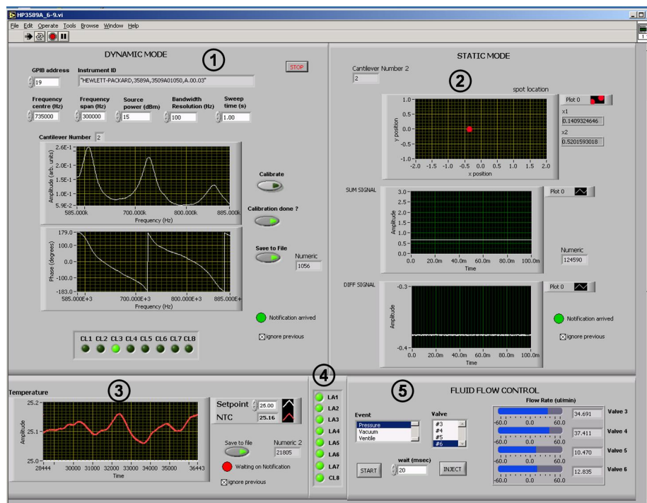
Fig. 2.8: Front panel of the combined mode setup. (1) Dynamic mode section, the amplitude spectra and phase spectra read from the spectrum analyzer, with possibility to choose center frequency, span and input excitation power. (2) Static mode section, the sum and difference signal for each signal. Only the signals from one of the cantilevers are displayed at a time. The laser position on the PSD can be visualized. (3) Temperature control of the box encasing the entire setup. (4) VCSEL selection. (5) Fluid flow control panel, by choosing vacuum or air, liquid flow rate can be controlled which is displayed
