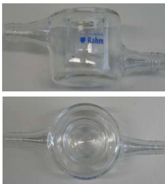
Fig. 1 Photos of a vessel used for controlling sample temperatures and measuring dielectric constants by immersing the dielectric probe in to the melted samples in this vessel.
