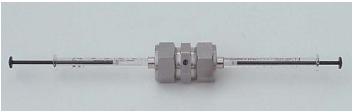
Figure 35: Hand-driven extrusion apparatus with a capacity of 1 ml (LiposoFast-Basic, Avestin, Ottawa, Canada). A 50 - 400 nm pore-size polycarbonate membrane is placed in the filter holder (middle). Back-and-forth passages of the sample between the two syringes result in a defined size of extruded liposomes.
