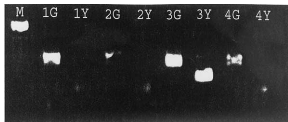
Figure 1. Analysis of total cell-free DNA and male fetal DNA in maternal urine by multiplex nested PCR. Total cell-free DNA was detected by a PCR assay for the ubiquitous \beta -globin gene (G). Male fetal DNA was detected by an assay specific for the SRY gene on the Y chromosome (Y). M = 25-bp DNA ladder molecular weight marker (Invitrogen). G = \beta -globin PCR product (240 bp); Y = SRY gene PCR product (133 bp). Samples 1 and 2 = amplification of urine samples from pregnant women carrying a male fetus. No Y-chromosome-specific DNA was detectable. Sample 3 = positive control from male genomic DNA, in which both globin- and SRY-specific signals were detected. Sample 4 = negative control from female genomic DNA, in which only the globin-specific amplicon was detected.
