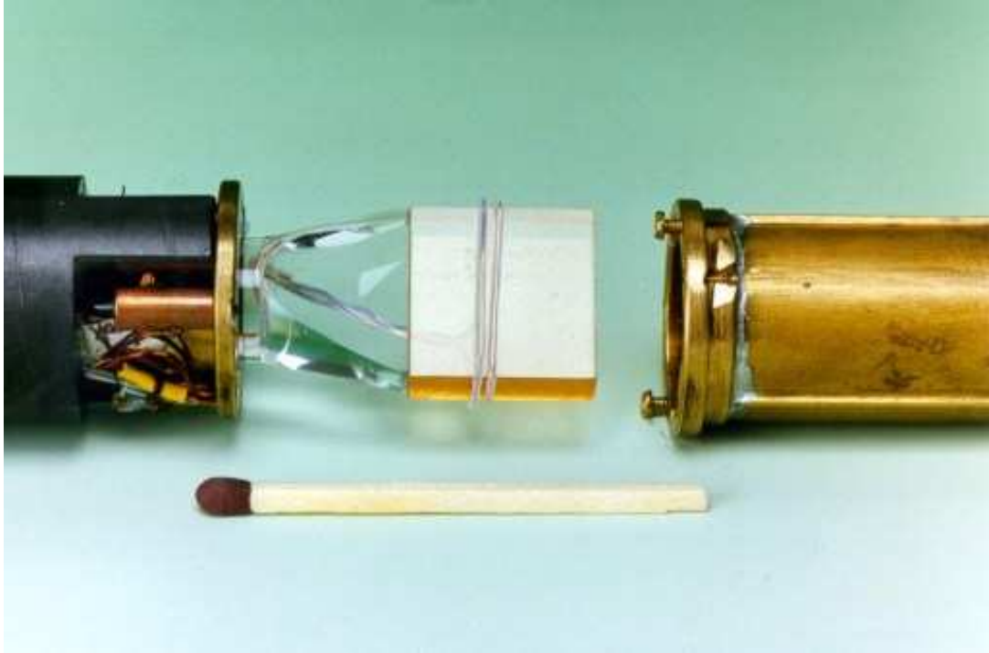
Figure 3: Sample of the polarizable active target and the NMR coil, mounted on the lower end of the PSI dilution refrigerator [18]
