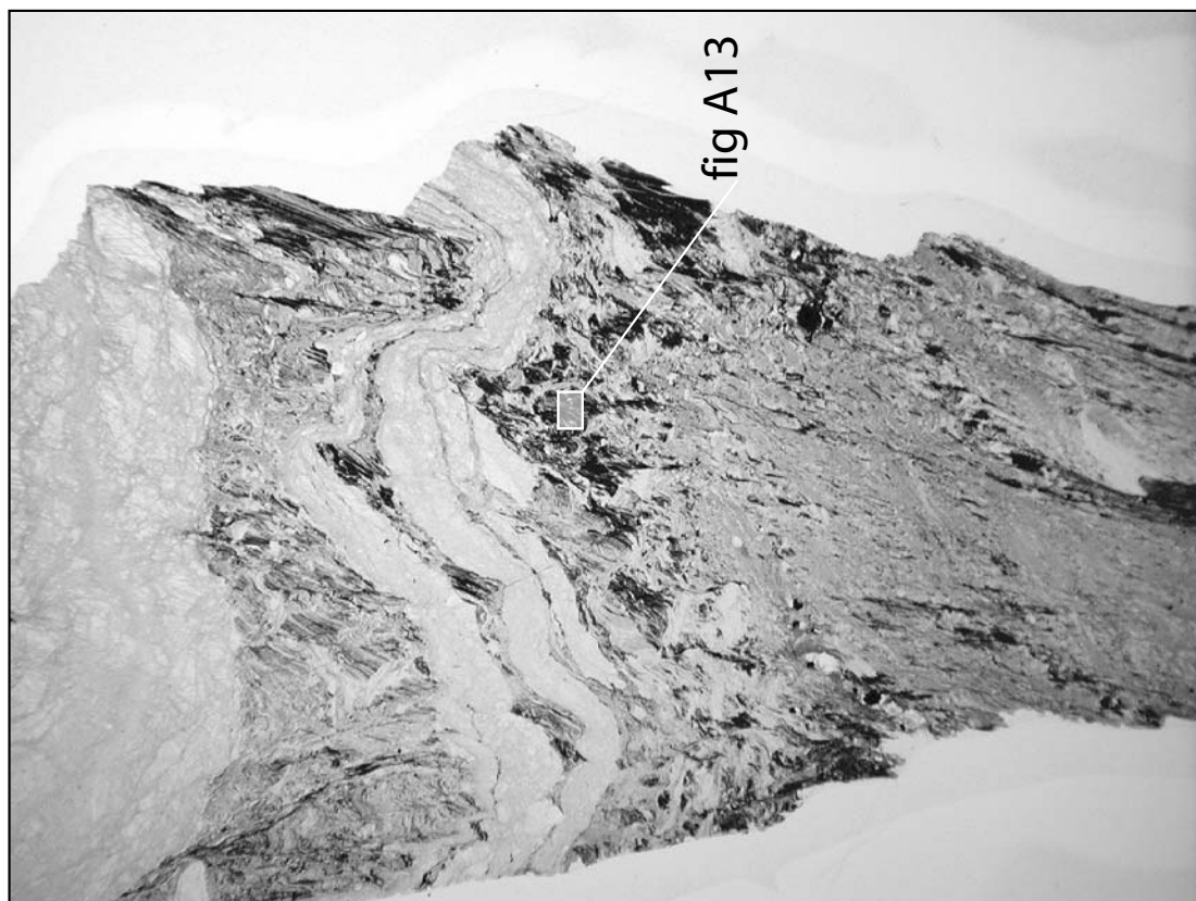
Figure A12: Micrograph interpretation of marl sample from outcrop depicted in figure A11. Note the superposition of two schistosities S0/1 and S2.
