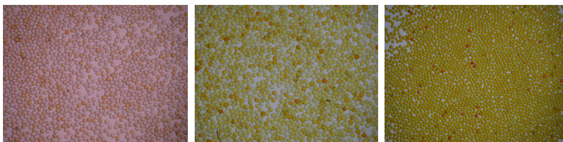
Figure 21: Screenings of the dye-marked receptor 46 in different buffers; a) 10 mM Tris·HCl buffer at pH 7.2 (left); b) 10 mM NaHCO 3 buffer at pH 8.5 (middle); c) 10 mM NaOH at pH 12.0 (right).
