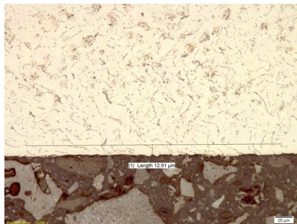
Figure G.25 - Grade 4 deformation depth at 0.25 mm DOC and 70 m/min
