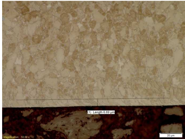
Figure G.38 - Grade 5 deformation depth at 0.25 mm DOC and 100 m/min
