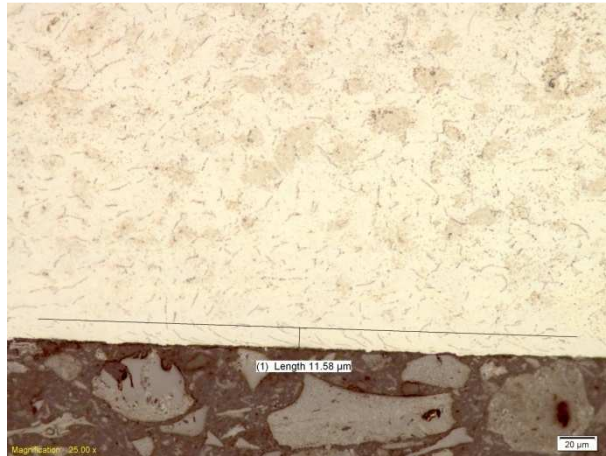
Figure G.26 - Grade 4 deformation depth at 0.25 mm DOC and 100 m/min
