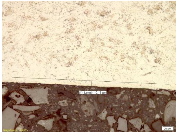
Figure G.29 - Grade 4 deformation depth at 0.25 mm DOC and 250 m/min
