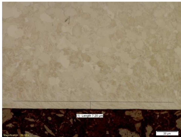
Figure G.45 - Grade 5 deformation depth at 1.00 mm DOC and 125 m/min
