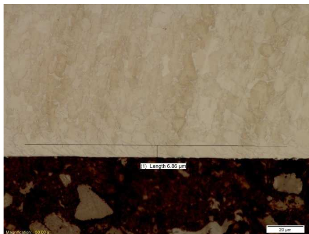
Figure G.46 - Grade 5 deformation depth at 1.00 mm DOC and 150 m/min
