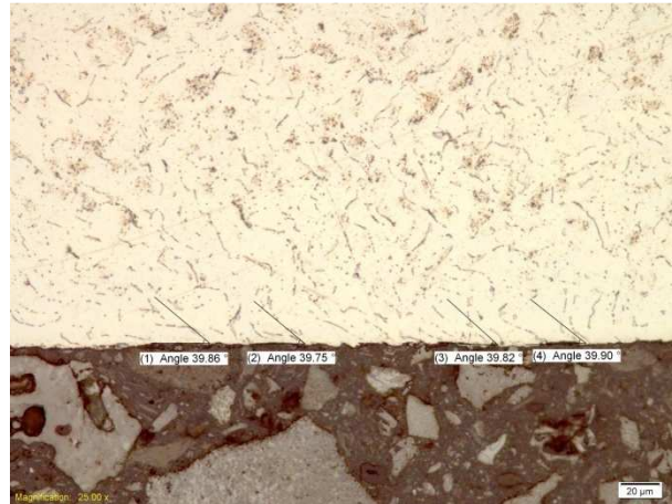
Figure G.5 - Grade 4 deformation angle at 0.25 mm DOC and 250 m/min
