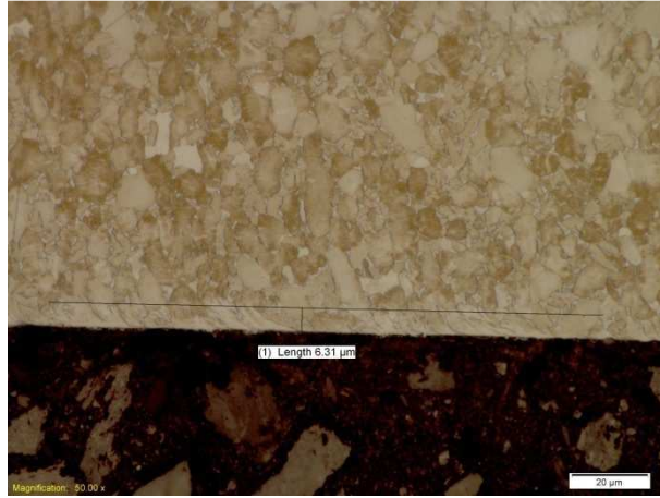
Figure G.47 - Grade 5 deformation depth at 1.00 mm DOC and 175 m/min
