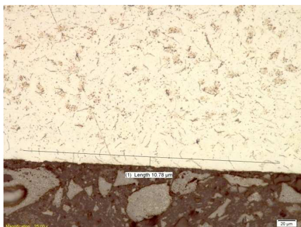
Figure G.28 - Grade 4 deformation depth at 0.25 mm DOC and 200 m/min
