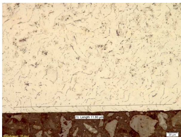
Figure G.31 - Grade 4 deformation depth at 1.00 mm DOC and 70 m/min
