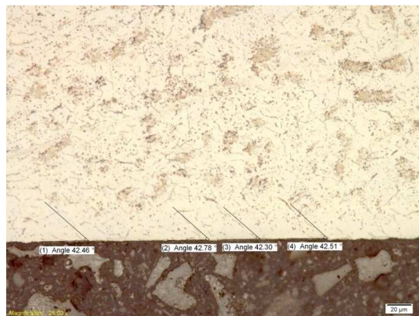
Figure G.6 - Grade 4 deformation angle at 0.25 mm DOC and 300 m/min
