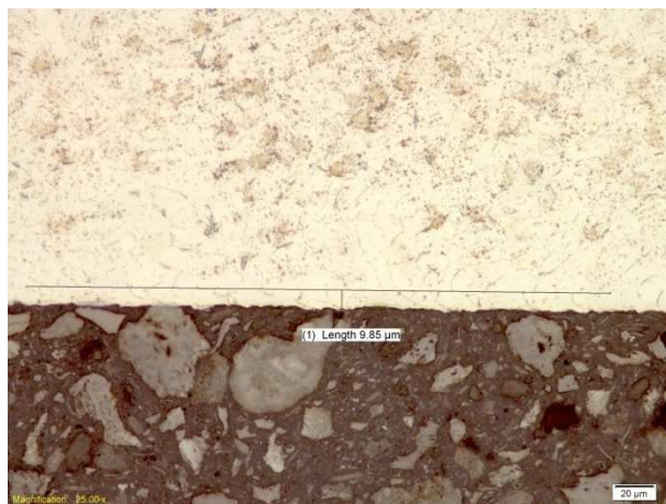
Figure G.30 - Grade 4 deformation depth at 0.25 mm DOC and 300 m/min
