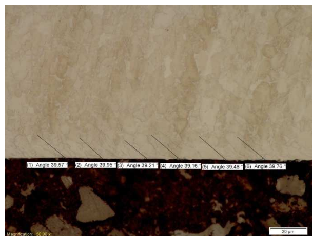
Figure G.22 - Grade 5 deformation angle at 1.00 mm DOC and 150 m/min
