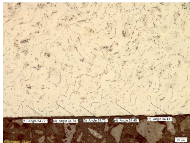
Figure G.7 - Grade 4 deformation angle at 1.00 mm DOC and 70 m/min
