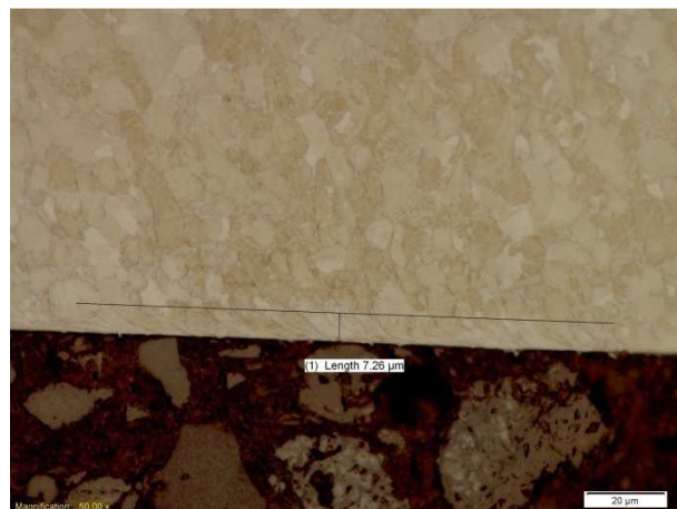
Figure G.37 - Grade 5 deformation depth at 0.25 mm DOC and 70 m/min
