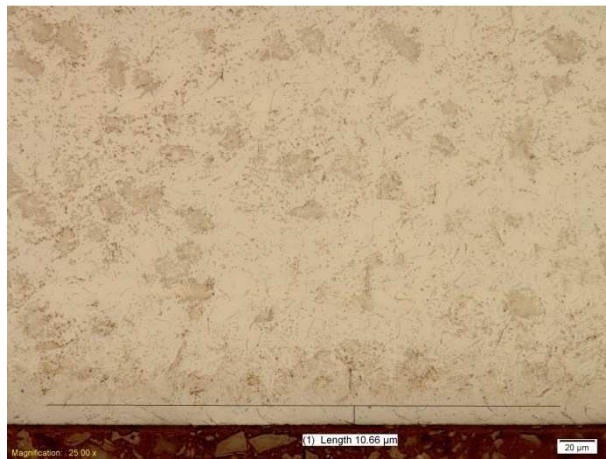
Figure G.33 - Grade 4 deformation depth at 1.00 mm DOC and 150 m/min
