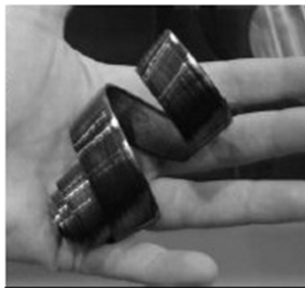
Figure 2.11 - Large chip created in high removal rate machining [93]
