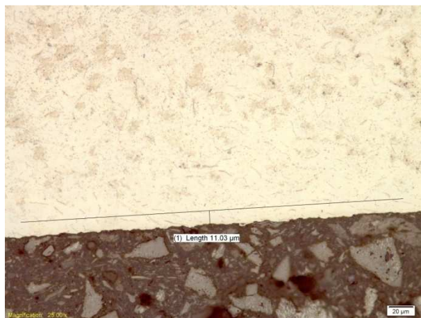
Figure G.27 - Grade 4 deformation depth at 0.25 mm DOC and 150 m/min
