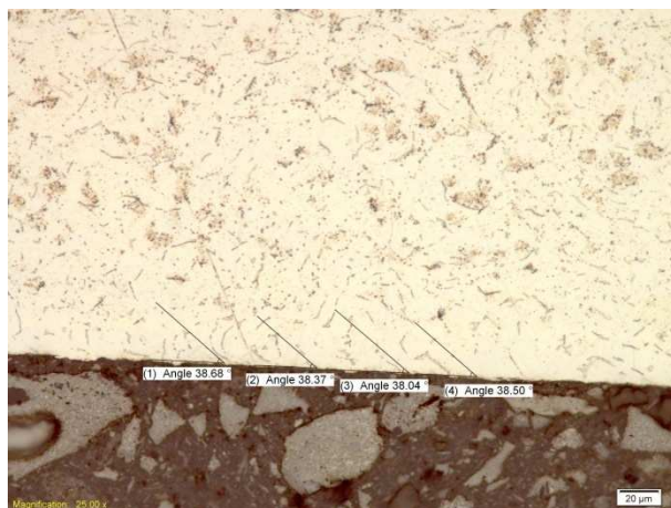
Figure G.4 - Grade 4 deformation angle at 0.25 mm DOC and 200 m/min
