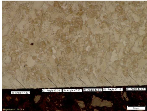
Figure G.17 - Grade 5 deformation angle at 0.25 mm DOC and 175 m/min
