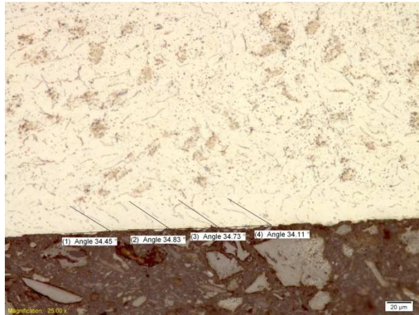
Figure G.2 - Grade 4 deformation angle at 0.25 mm DOC and 100 m/min
