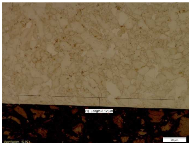
Figure G.43 - Grade 5 deformation depth at 1.00 mm DOC and 70 m/min
