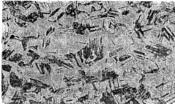
Figure 24. Optical micrograph of strain induced martensite in a Smartbolt™ alloy
