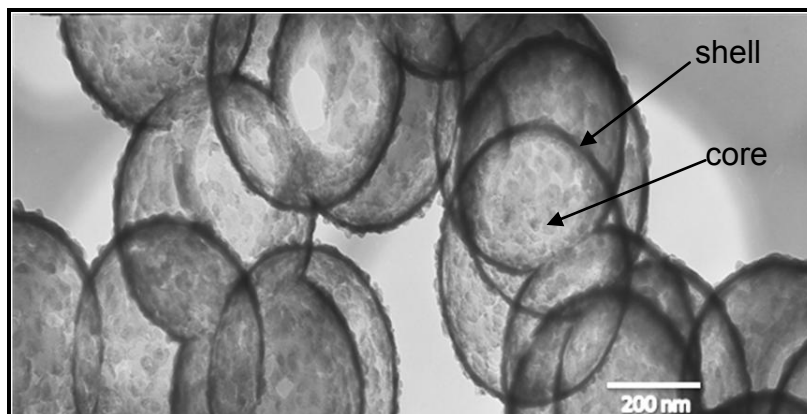
Figure 3.2: TEM image of oil loaded ALG/CS nanoparticles: magnification x50 000
