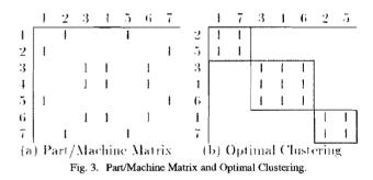
Although the array-based clustering techniques used in the design of manufacturing cells are both efficient and simple to apply to the part/machine matrix, there are still some
