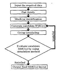
Fig. 4. Flow chart of RMC formation procedure.
