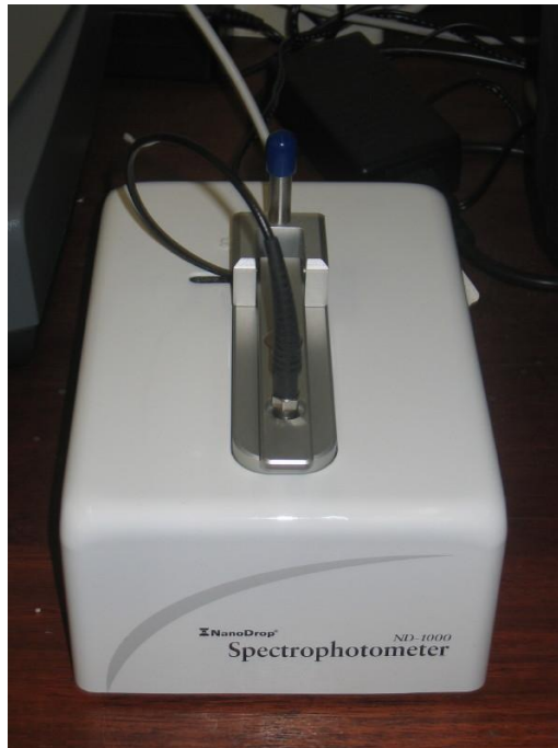
Fig. 2.3 – The Nanodrop 1 000 spectrophotometer used to determine the DNA concentration after DNA isolation (NanoDrop Technologies, Wilmington, Delaware USA).
