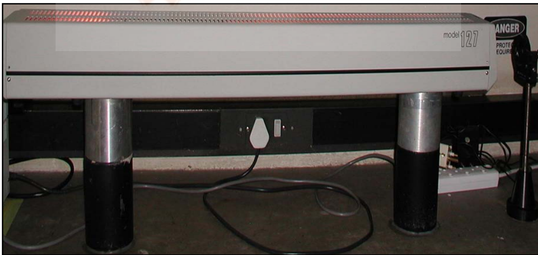
Figure 4 A He-Ne laser (Spectraphysics, model 127) was used to irradiate cells at \lambda 632.8 nm. This laser has a spot size of 9.08 cm 2 . He-Ne gas is the amplifying medium in this laser.
