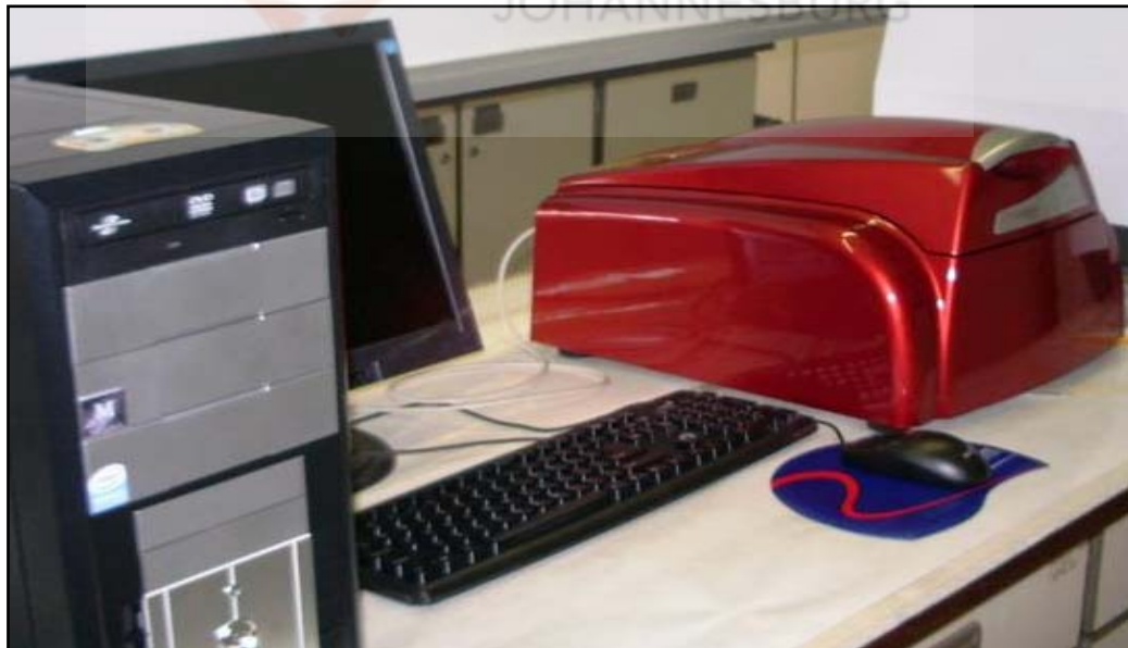
Figure A7 The RotorGene thermocycler which was used for the real time RT-PCR. It has a hardware for high resolution melts (HRM) which characterises samples based on sequence length, GC content and complementarity.
