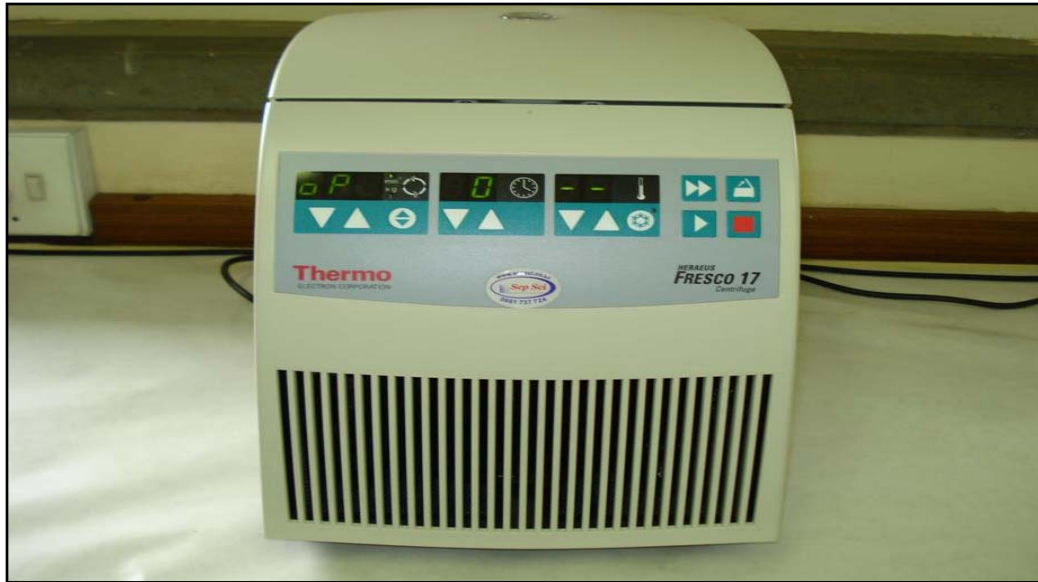
Figure A6 A centrifuge used to spin samples during RNA and cDNA synthesis. This centrifuge has both rpm and gravitation functions.
