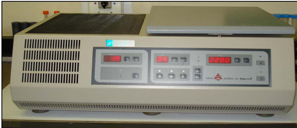
Figure A3 A centrifuge (DIGICEN-R, INSTRULAB S.A) used to spin cell culture suspensions at 2,200 rpm for 4 min.
