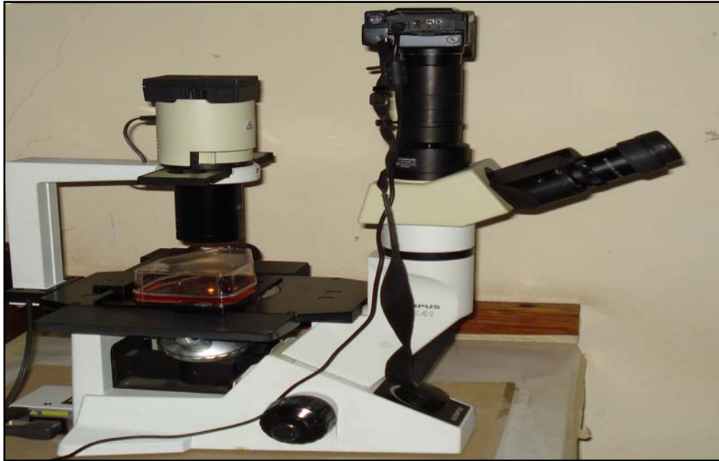
Figure A4 An inverted light microscope used to study cell morphology, check contamination and confluence of cells in the 75 cm 2 culture flasks and 3.4 cm diameter culture dishes. The microscope has a camera attached for digitally recording photographs.
