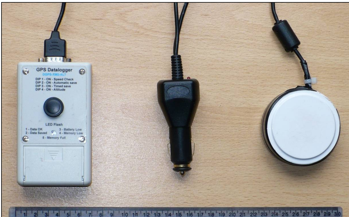
Figure 3.7: GPS datalogger (left), adapter for cigarette lighter sockets (middle) and GPS sensor (right).
