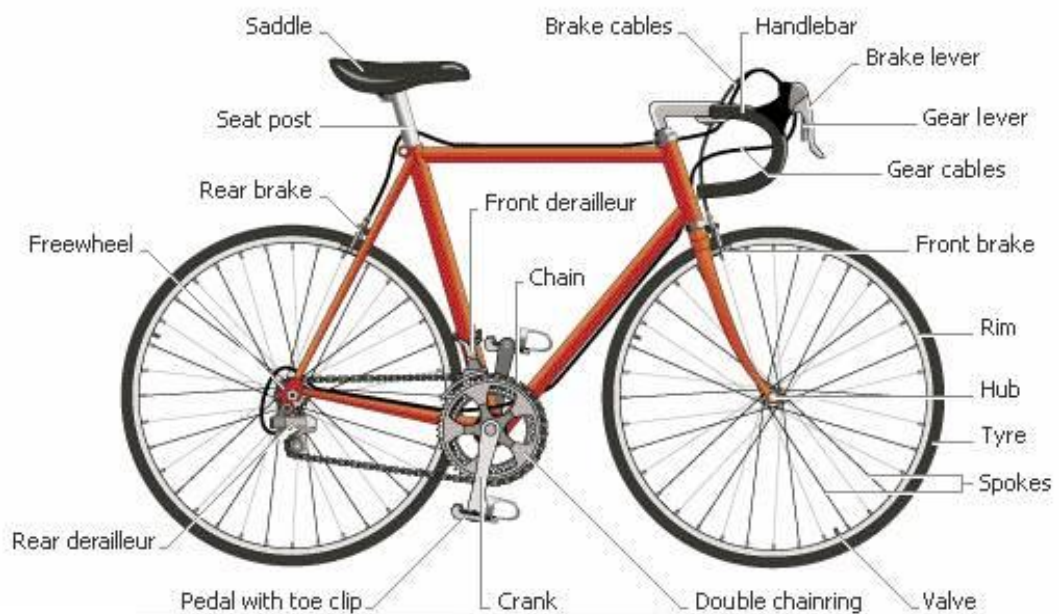
Figure 1: The Structure of the Bicycle (Microsoft Encarta Online Encyclopaedia 2005)
