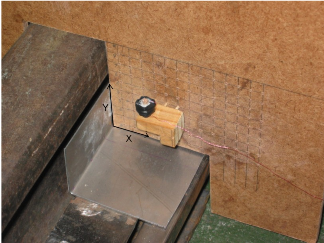
Figure 2-4: Test rig placed around railway track, showing metal shield and magnetic Flux Density Sensor and mounting.
