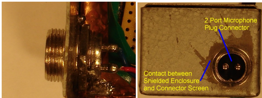
Figure 4-13: 2 Port Microphone Plug connector mounted to the chassis of one of the shielded enclosures, Top view on the Left with a front view on the Right.
