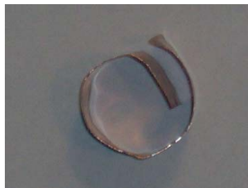
Figure 4-5: Copper sheet used for the shield of the Flux Density Sensor
