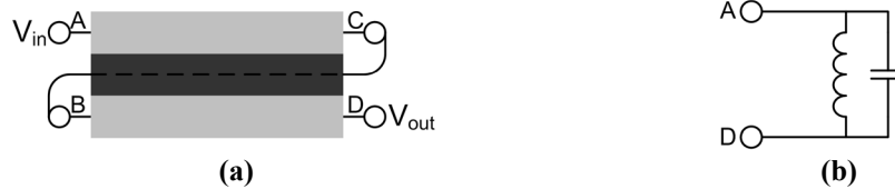
Fig. 1.4: (a) Parallel resonant configuration as realised with a two-layer IPPM (b) Equivalent circuit
