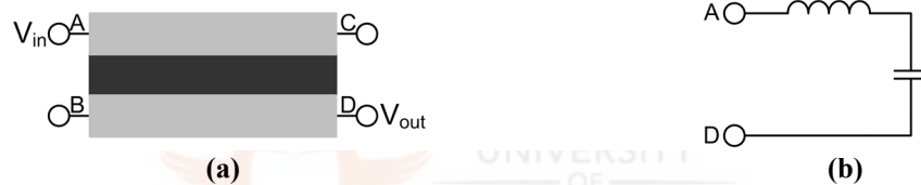
Fig. 1.5: (a) Series resonant configuration as realised with a two-layer IPPM (b) Equivalent circuit
