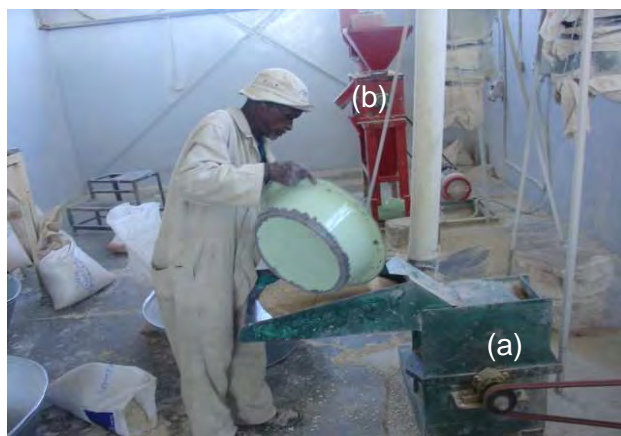
Figure 1. PRL-type Abrasive decorticator (a) and hammer mill (b) similar to those used to produce abrasive decortication-hammer mill meal samples.
