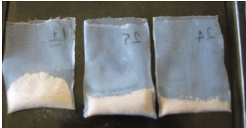
Fig. 13. Comparing coarse particles retained in pouches
