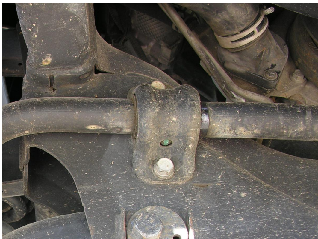
Figure 12. Roll Bar and Connecting Pin Damage, Test No. PCMB-1
