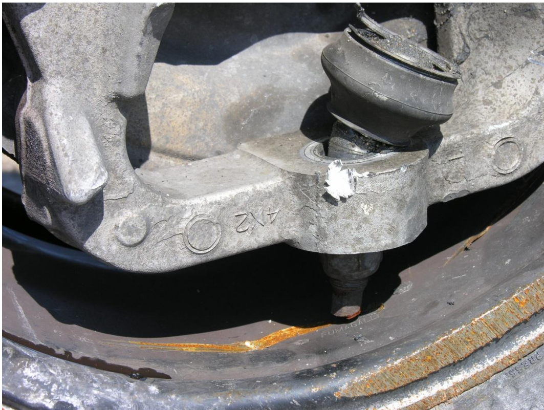
Figure 7. Inside of Wheel Damage, Test No. PCMB-1
