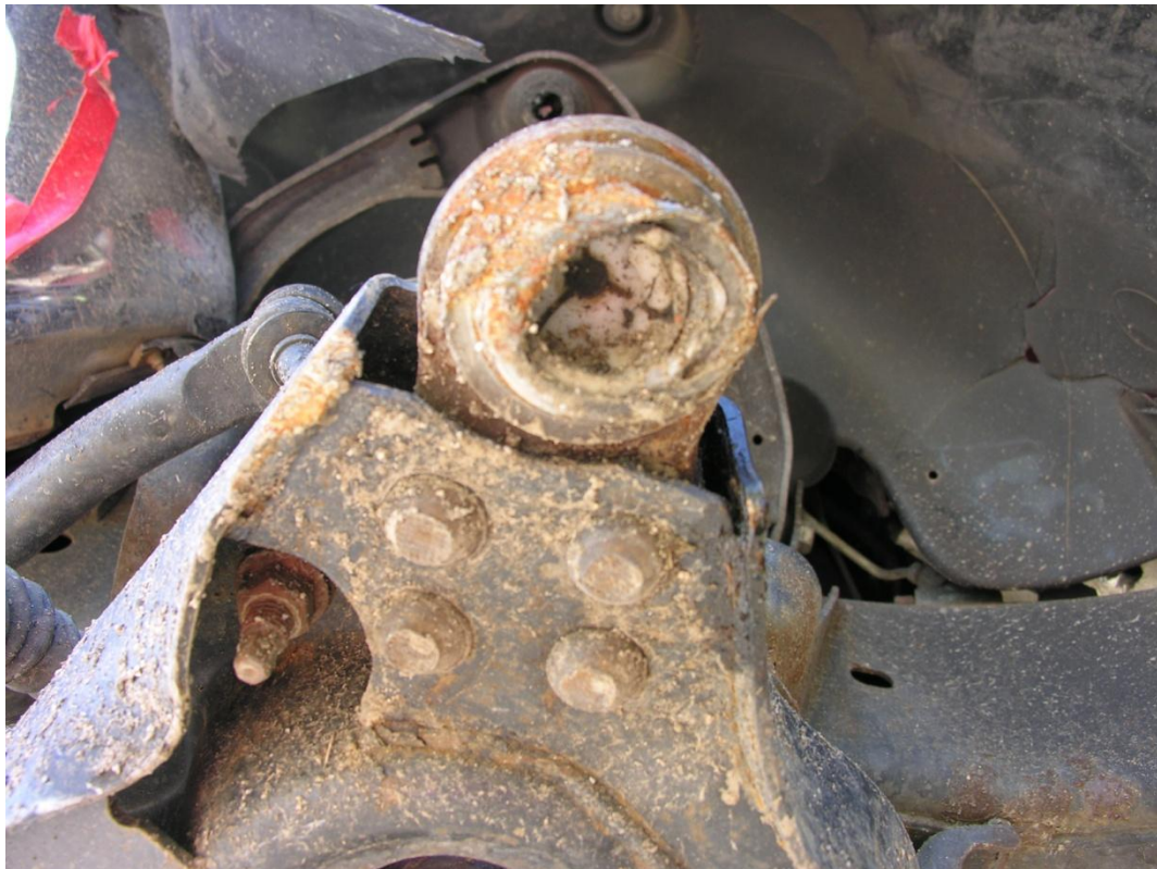
Figure 9. Lower Control Arm Damage, Test No. PCMB-1
