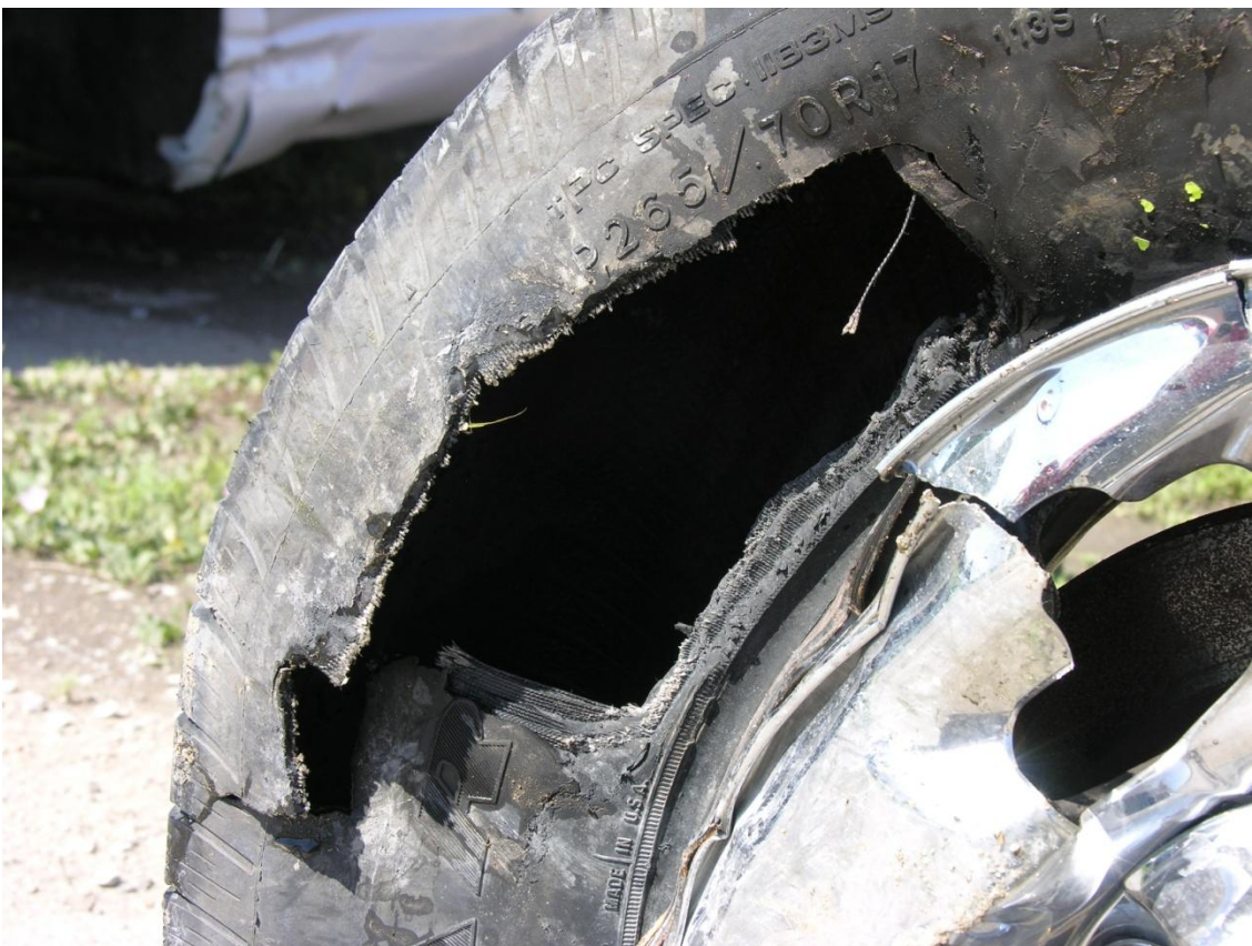
Figure 8. Outside of Wheel Damage, Test No. PCMB-1
