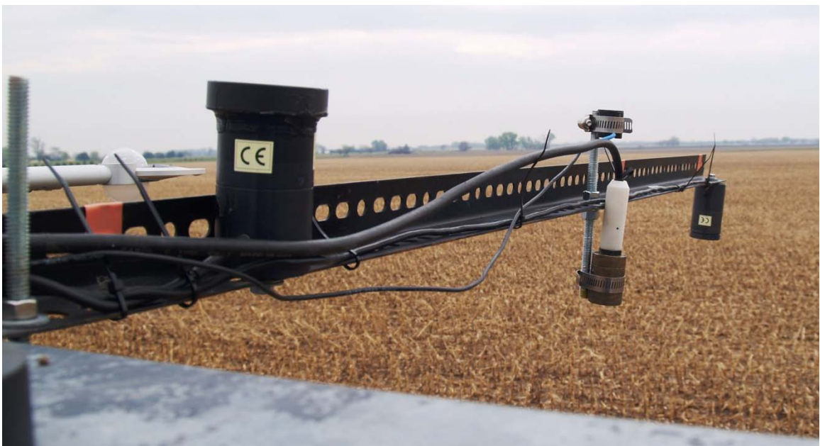
Figure 2.4: SKYE instruments mounted on the radiation tower over maize (Above) and a close-up image of the sensors (Below)
