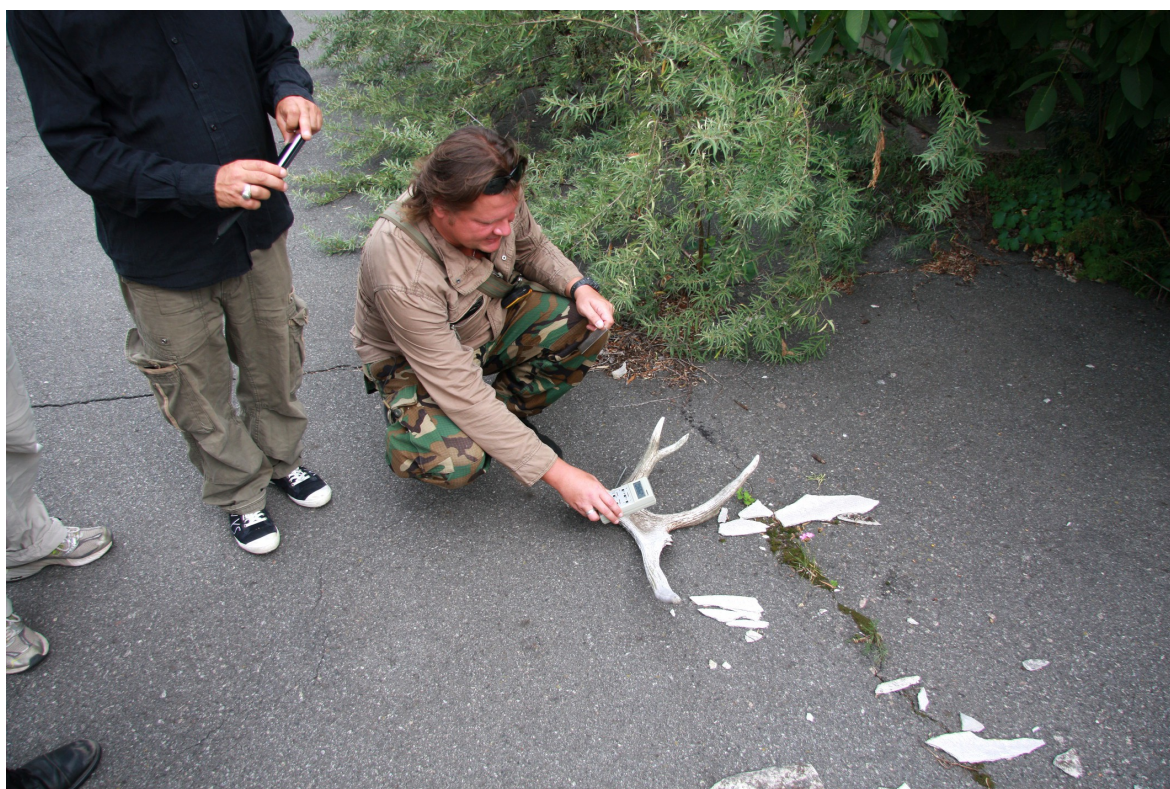
Image 60: Antler with ^{90}\text{Sr} contamination showing \beta -decay radiation, but not \gamma (#p1267)
