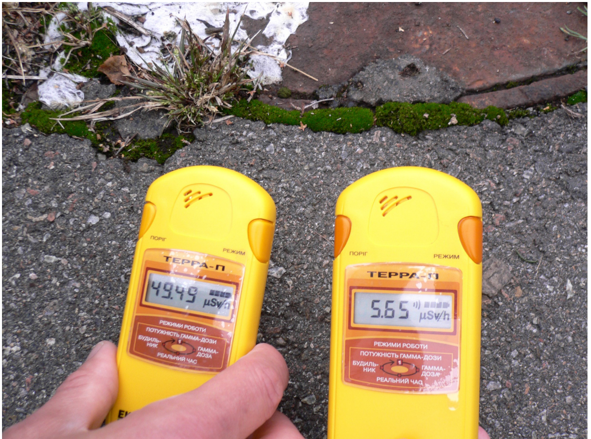
Image 58: (Close up of patch of asphalt in above image) In comparing my counter (right) with that held by visitor (left) which has had the \beta -particle barrier removed, it is clear that the patch of asphalt above is almost entirely a source of \beta radiation (meaning it is likely ^{90}\text{Sr} in the asphalt, though also possibly an isotope of Plutonium) (#p1762)
