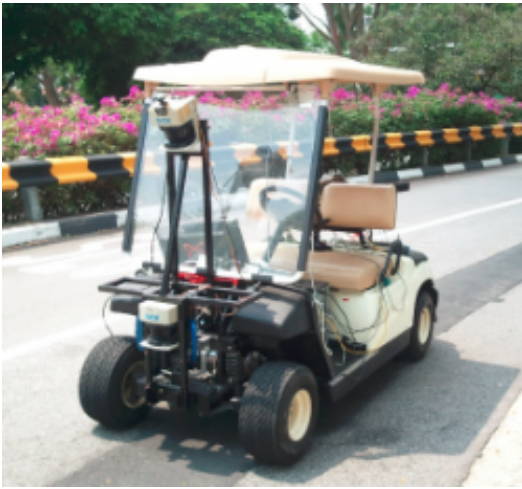
Fig. 8. Yamaha G22E golf cart mounted with various sensors
