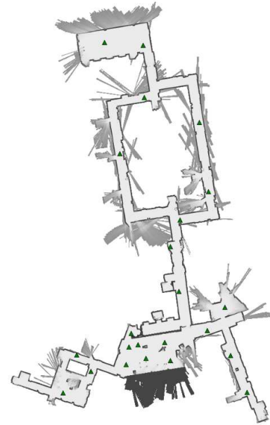
Figure 4: Candidate destinations. Destinations (triangles) are proposed by using spectral clustering on the graph of the RRG.
