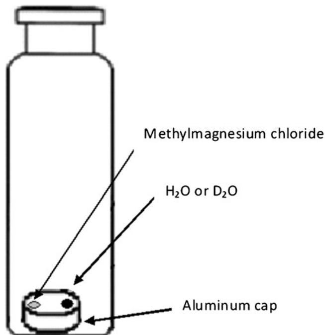
**Fig. 1** Design of methane generation in situ
