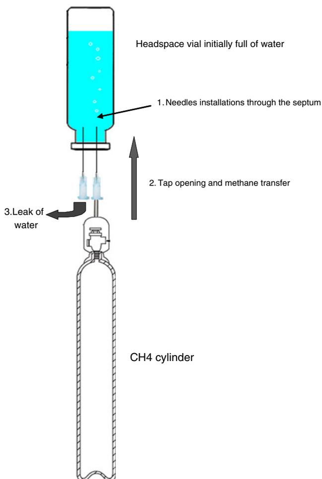
**Fig. 2** Design of methane transfer to perform external control samples
