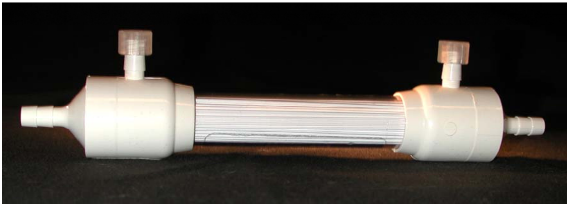
Figure 5.2: Picture of the hollow fiber module 1 made of hydrophilic polyethersulfone fibers with a diameter of 0.5 mm, ECS volume of 25 ml, fiber surface area of 420 cm 2 and porosity of 0.5 μm. The hollow fibers are bundled together within a transparent plastic shell.
