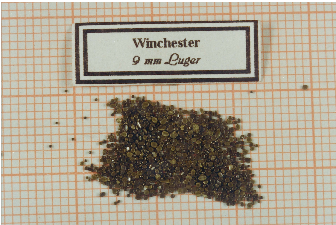
Fig. 7. WINCHESTER 9 mm Luger cartridge with SUPER-X ® SUPER UNLEADED primer.
