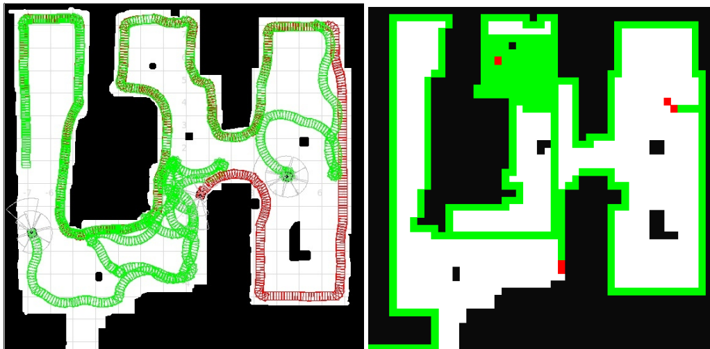
Figure 7.5: TeSLiSMA algorithm by Player/Stage (right) and CLOWN formalism (left)
